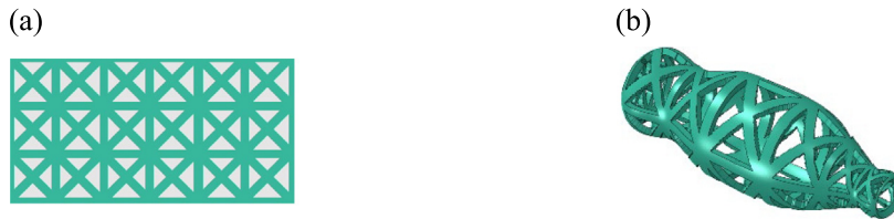
Fig. 21. Initial layout of components. (a) In the parametric domain. (b) On the original thin-walled structure.
