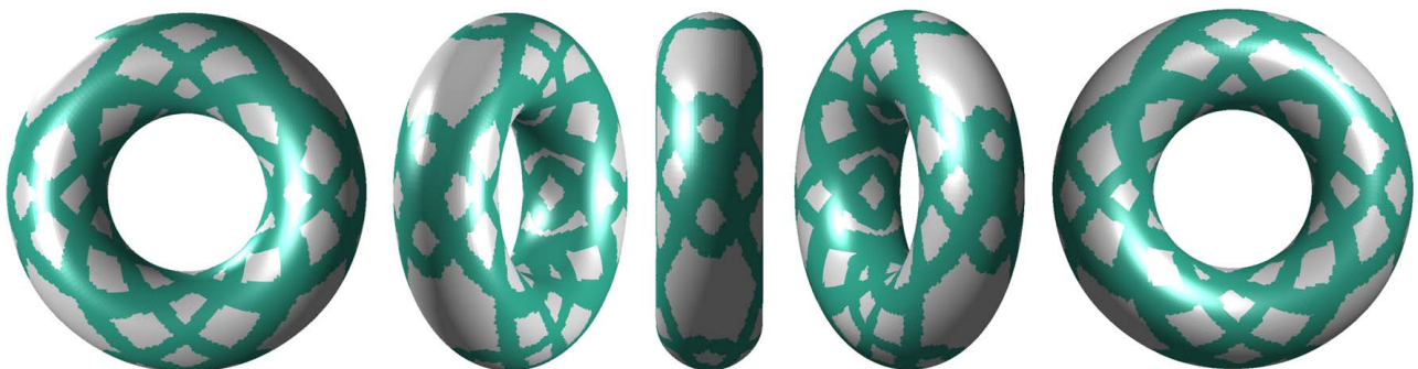
Fig. 16 The optimized design of the torus surface example (viewing from different directions)
